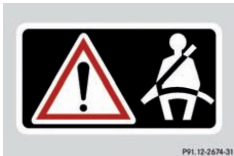
Warning symbol on the connector of the rear seat belt status indicator
